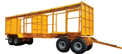
4 axles platform drawbar trailer Modified for sugarcane Transport
