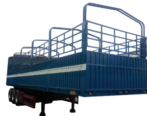
3 Axle Drawbar trailer with dropside doors & Extended poles for tarpaulin cover
